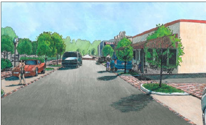
Fort Thompson Avenue after the proposed streetscape improvements: street trees and landscaping have been added, sidewalks have been widened and improved, café seating has been added under covered walkways, and onstreet parking has been clearly designated along the sides of the streets.
